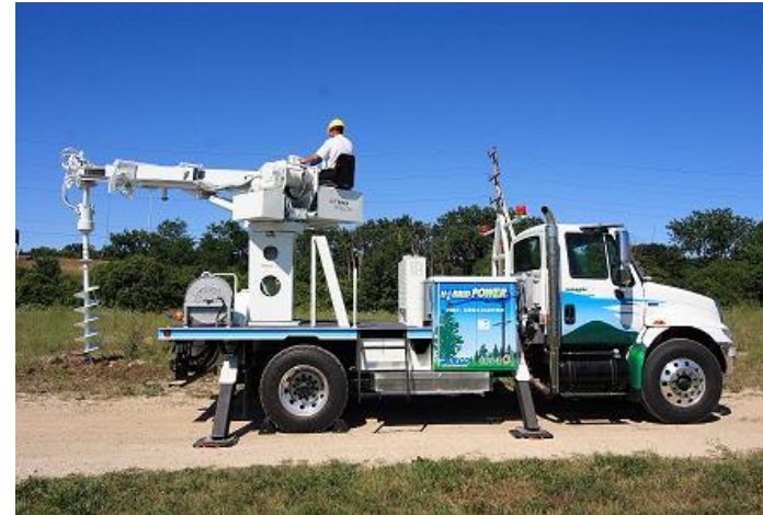
Hybrid Digger Derrick
